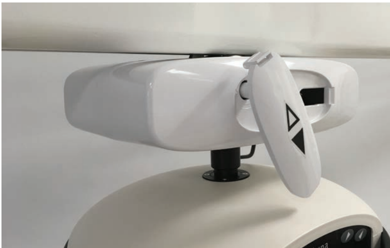
The patented integrated safety release handle allows manual transfer if needed
