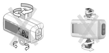
We do not recommend building a scale into a construction of any hoist where the spreader bar do not swivel 360°.
